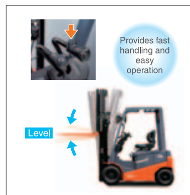
Automatic Fork-leveling Control
